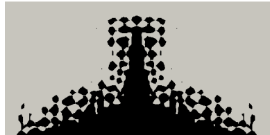
Fig. 16: Convective design resulting from no feature size enforcement ( c_{MN} = \infty ).
