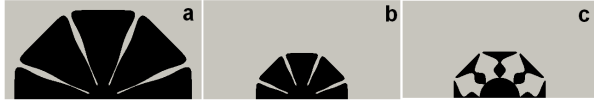
Fig. 15: Comparison of optimized designs for B = 0.1 : (a) unconstrained, (b) perimeter constrained, and (c) volume constrained.
