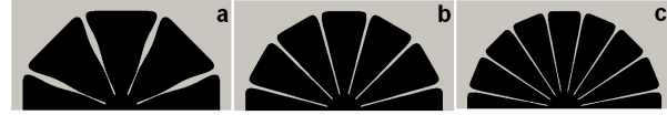
Fig. 14: Comparison of designs for varying numbers of petals at B = 1.0 : (a) 5 petals, (b) 7 petals, (c) 9 petals.
